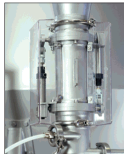
Fine powder recycling through double flap valve and swirl valve.
